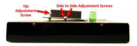
Bracket can be mounted slightly tilted or cocked to one side
